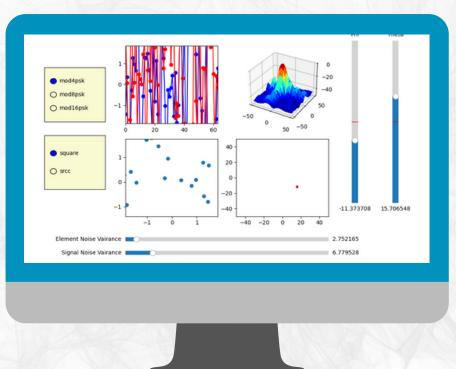
Python code to illustrate and explore the design space of signal Angle-of-Arrival (AoA), based on IQ samples and the Bartlett algorithm, using planar antenna arrays. A planar array is composed of homogeneous antenna elements, which all receive replicas of a given signal.
